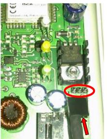
state. Start the gateway first and wait for network log in. Then connect cable from ACU pack to appropriate connector..
