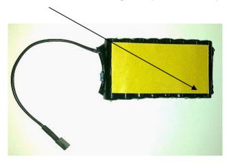
3. Fix the ACU pack into Gateway cabinet. CAUTION for holes for signalling LEDs! DO NOT COVER!
