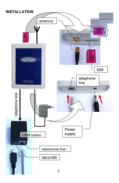
Insert the SIM card up the picture and by press fix it in operation position. Before inserting the SIM card we recommend checking at various mobile phone state of the SIM card (logging with or without PIN, PIN, etc.) and set logging without PIN. When you want logging with PIN you have to preprogrammed this PIN and set logging with PIN (via table of programming). Without this setting the Gate wont work.
