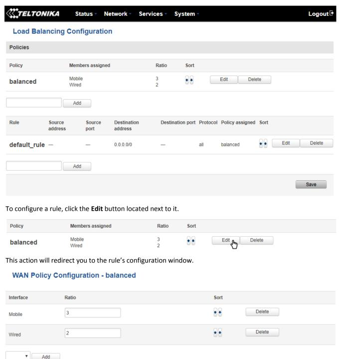
Here you can define the ratio of each WAN interface. In the example above we can see that the mobile interface's ratio is 3, and the wired interface's ratio is 2. This means that  $\frac{3}{5}$  of all traffic will go through the mobile interface, and  $\frac{2}{5}$  will go through the wired interface. After you've finished configuring you Load Balancing rules, go the WAN section and activate Load Balancing for the desired interface.
