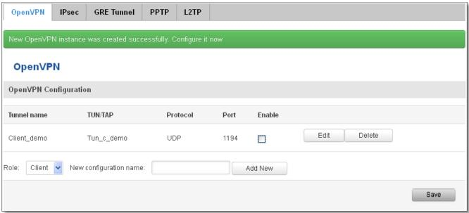
To see at specific configuration settings press "edit" button located in newly created configuration entry. A new page with detailed configuration appears, as shown in the picture below (TLS client example).
