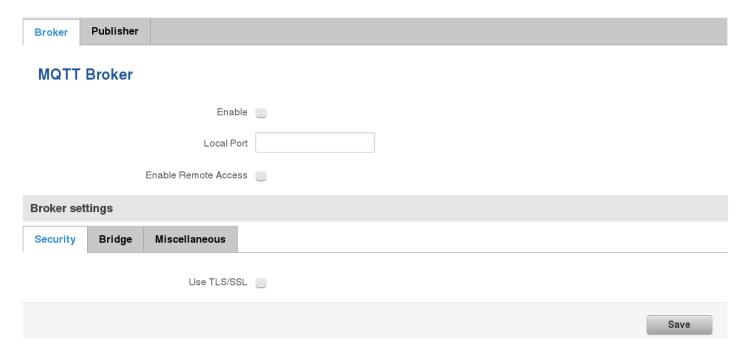
In order to use TLS/SSL for connecting clients (subscribers and publishers) to the broker, the one should check *Use TLS/SSL*. After that, additional settings will be displayed to the user as shown below. Here the user can upload certificates, key files and choose TLS version, which will be used for data encryption between broker and clients (subscribers and publishers)
