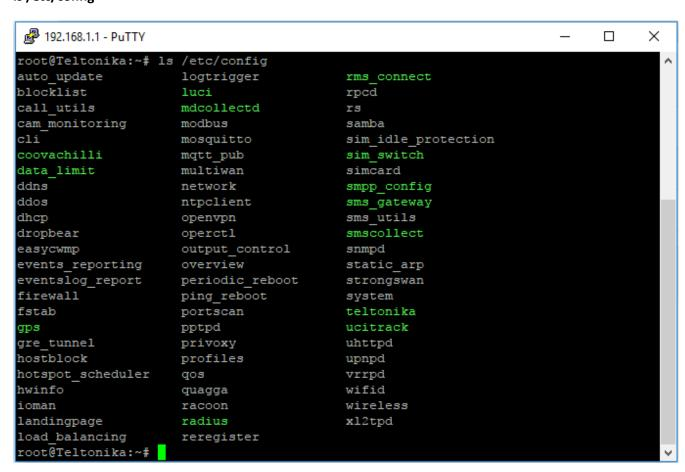
You can use the **cat** command to view the contents of a file. For example, to view the contents of the **network** config, you should use this command:
