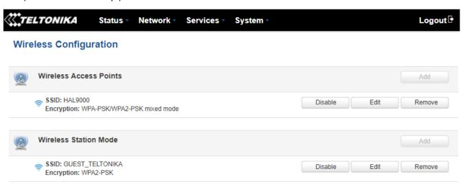
Above is the overview of the Wireless Configuration window. It displays active access points and stations. Here you can disable or enable your Wi-Fi interfaces, remove unwanted access points or stations or enter a configuration window for each Wi-Fi, where you can configure it more thoroughly.
