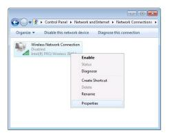
6. By default the router is going to have DHCP enabled, which means that if you select "Obtain an IP address automatically" and "Obtain DNS server address automatically", the router should lease you an IP and you should be ready to login.
